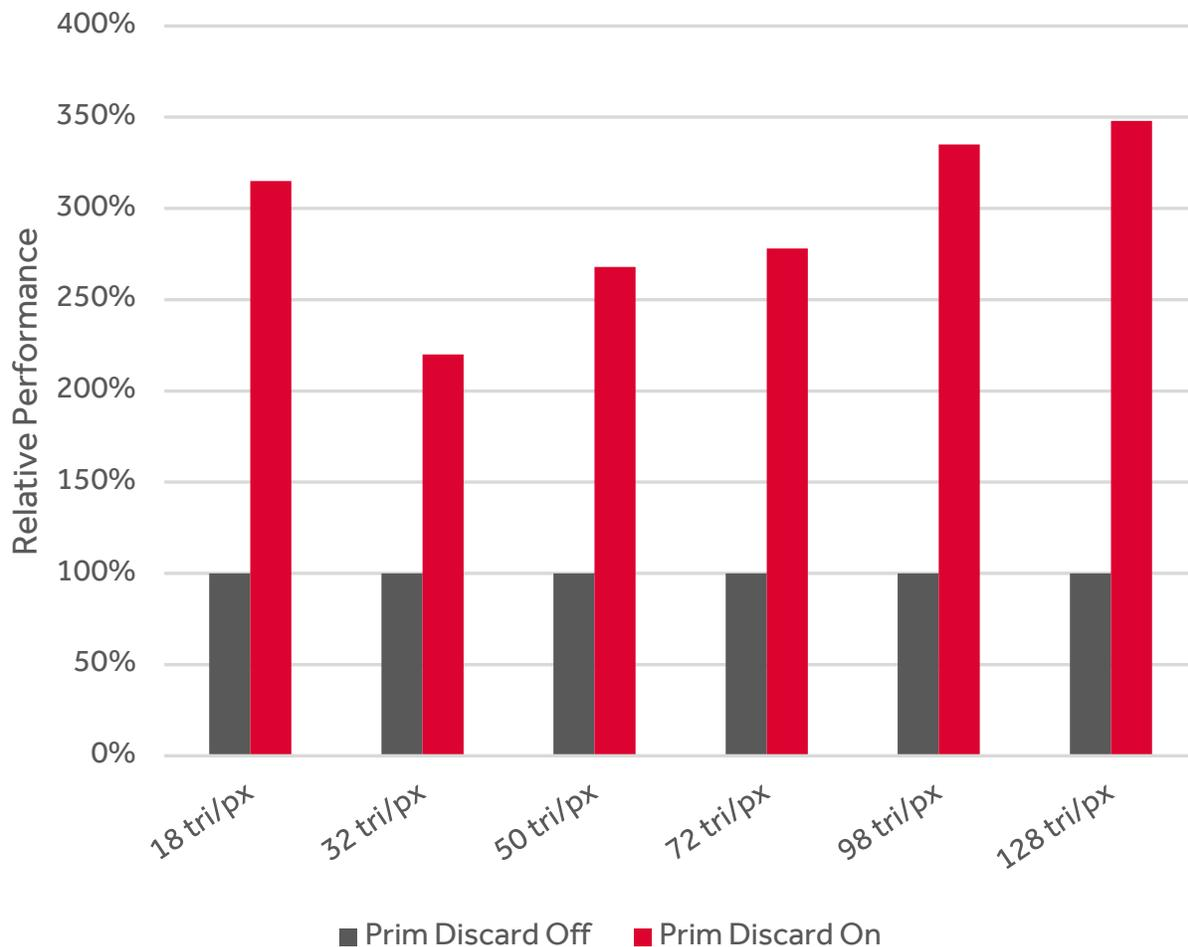
**Figure 6:** The primitive discard accelerator for small and degenerate primitives is more effective as the triangle density increases.<sup>2</sup>
