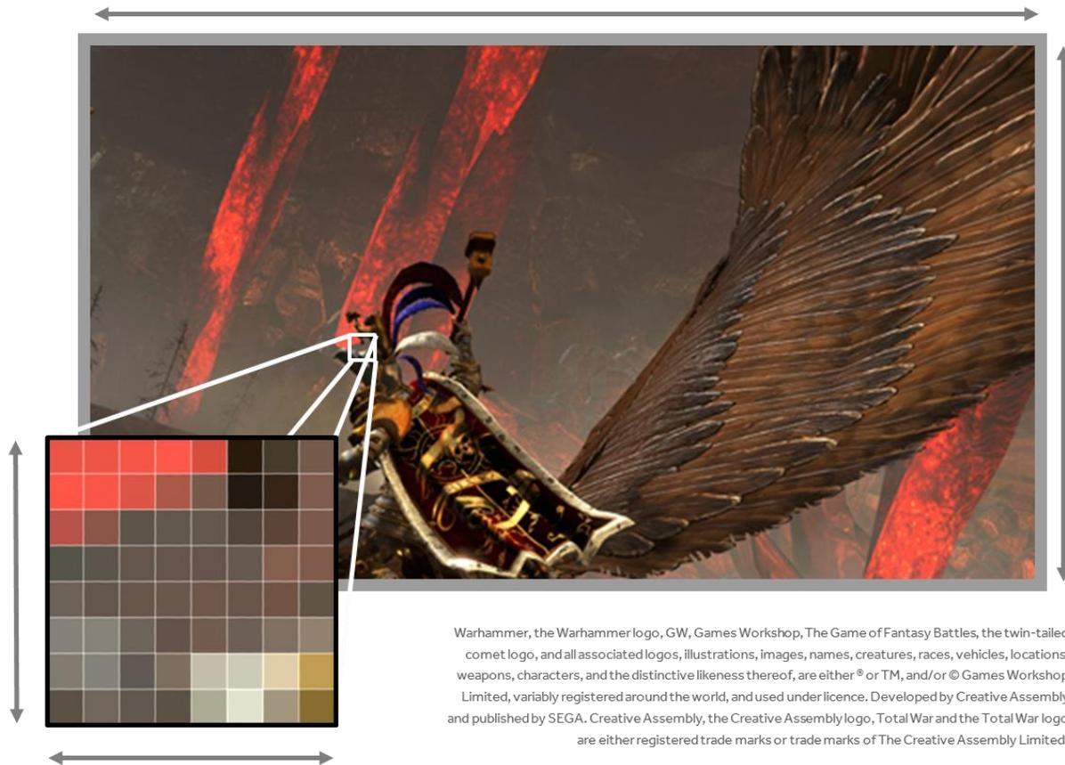
**Figure 15:** A new two-pass VBR encoding mode on the Polaris architecture analyzes the frame and macroblocks in the scene during a pre-encode pass to intelligently guide bitrate and QP selection during final encode.
