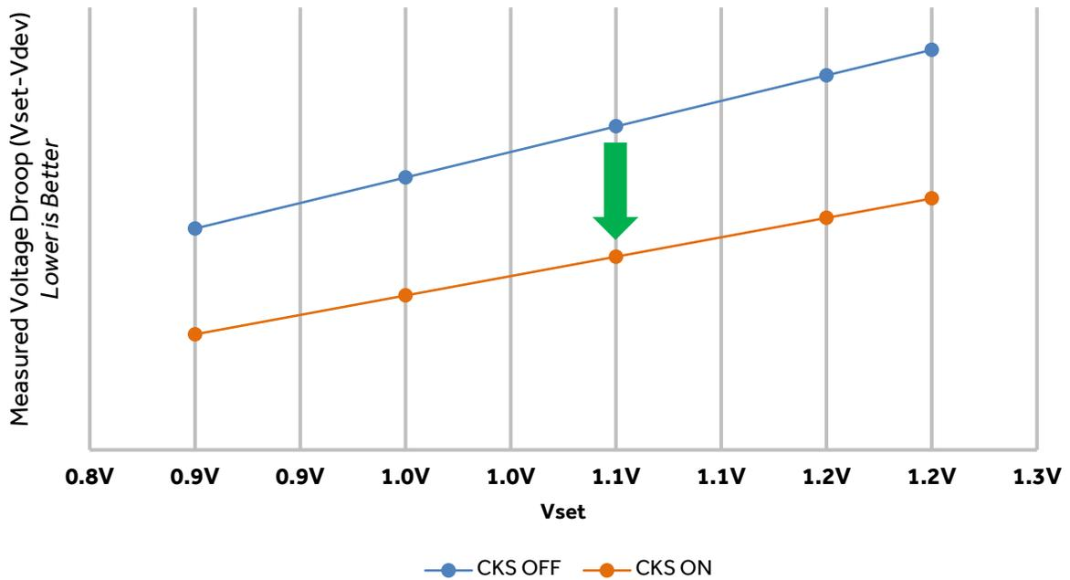
*Figure 10: AMD's adaptive clocking technology mitigates voltage droop events, which enables up to 140MHz higher frequency in the Radeon™ RX 400 Series GPUs based on the Polaris architecture.*
