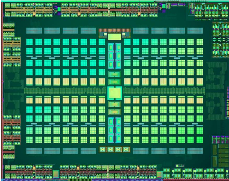
Figure 1: Die plot of the Radeon™ RX 480 GPU, which is based on the Polaris architecture.
