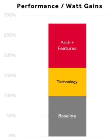
**Figure 16:** the FinFET 14 process proves a solid foundation for the energy efficiency of the Polaris architecture, but AMD proprietary power management and circuit design techniques were pivotal in extracting peak performance per watt.
