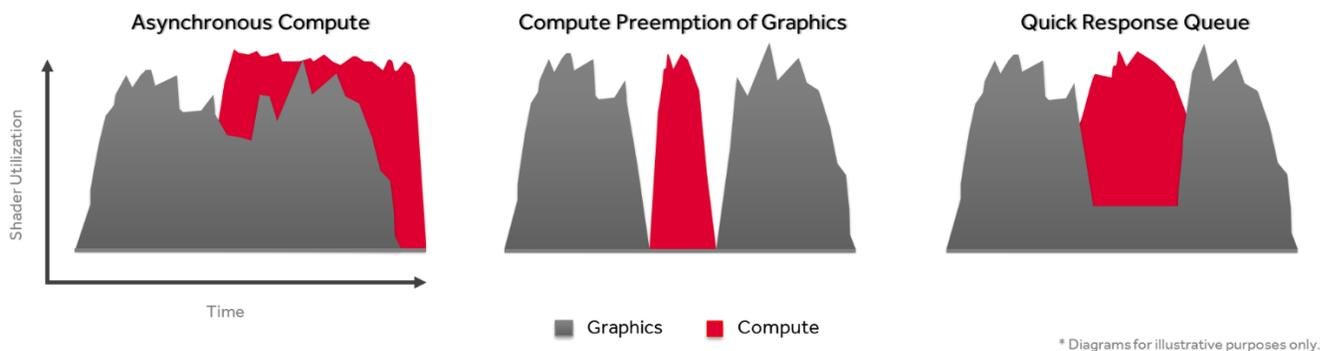
**Figure 3:** The Polaris architecture can use its advanced asynchronous compute capabilities in many ways, including compute/graphics concurrency (left), compute preemption of graphics (middle), and compute QoS (right) for latency-sensitive tasks.
