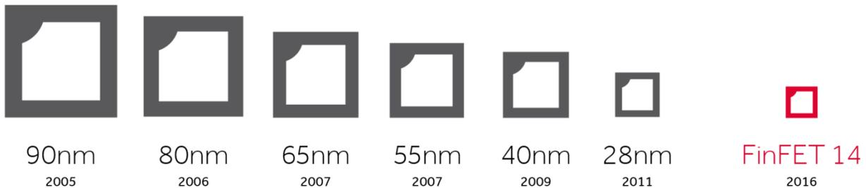
Figure 2: Evolution of process nodes utilized by Radeon™ graphics since 2005.
