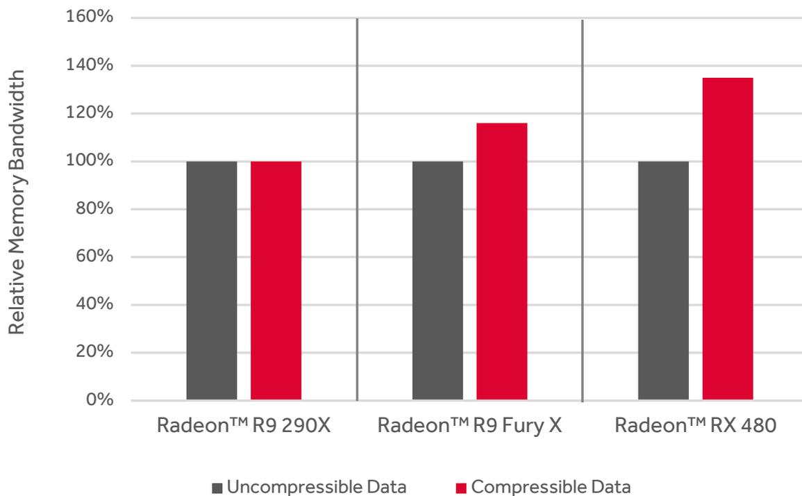
*Figure 7: The efficacy of AMD's delta color compression technology has increased over time, increasing the effective memory bandwidth up to 35% on the Radeon™ RX 480 with the Polaris architecture.<sup>3</sup>*
