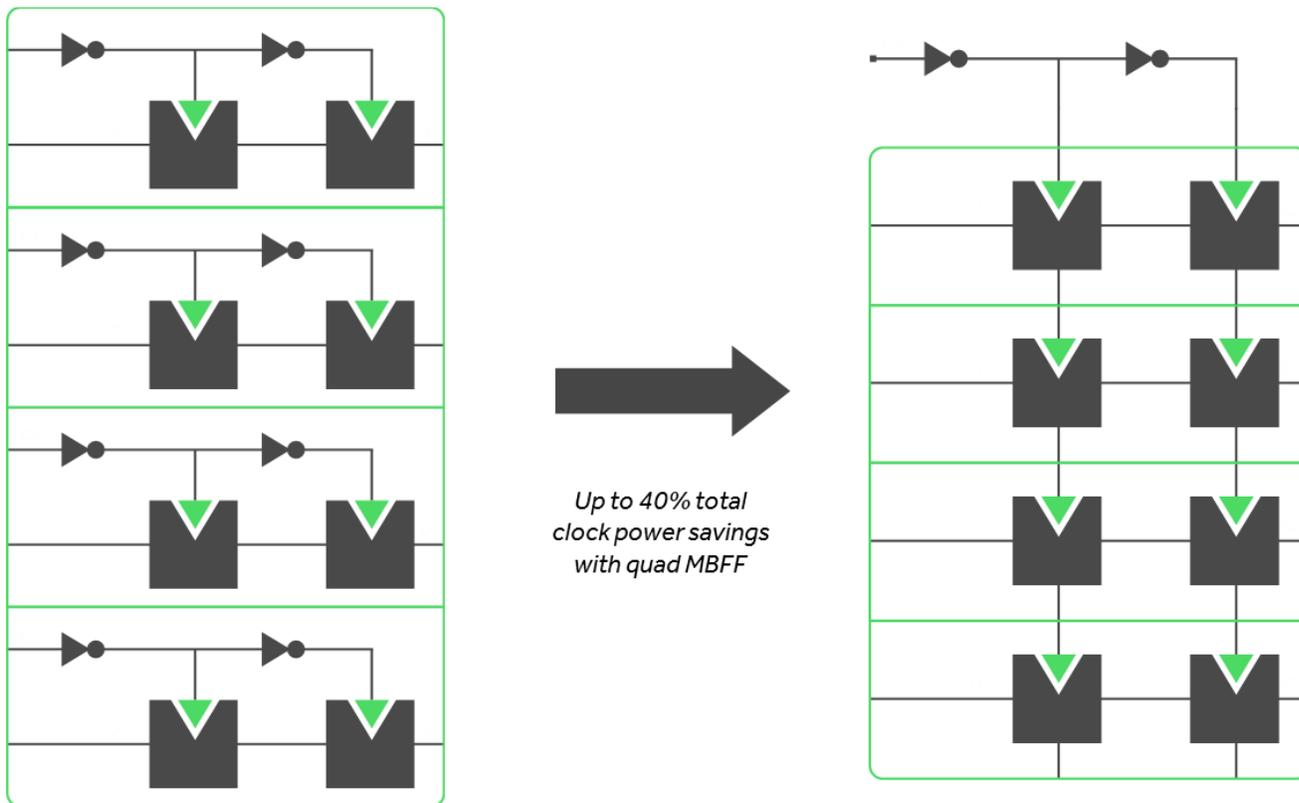
**Figure 11:** The structure of a set of normal flops (left) vs. quad MBFF used in the Polaris architecture (right). The quad MBFF reduces die area, reduces clock power by up to 40%; and generally reduces total product TDP by 4-5%.
