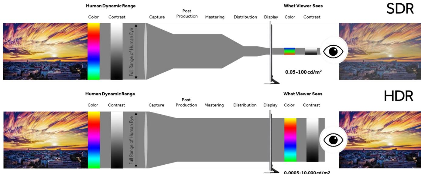
**Figure 14:** HDR capture, mastering, distribution and playback attempts to capture a significantly wider portion of the human visual system. The result is a significantly more lifelike image.
