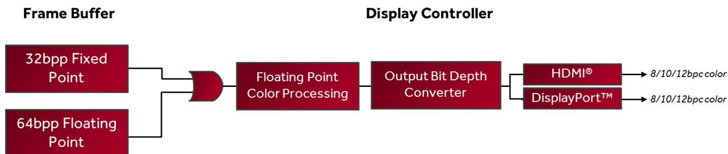
*Figure 13: The display pipe on the Polaris architecture can handle 32bpp fixed point or 16bpp floating point framebuffer data, allowing for 8/10/12bpc output to HDMI® or DisplayPort™ displays.*
