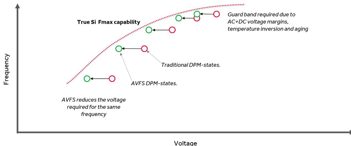
**Figure 9:** AVFS in the Polaris architecture permits the reduction of voltage/frequency margin that would "leave performance on the table", improving performance and energy efficiency in products. (Diagram for illustrative purposes.)
