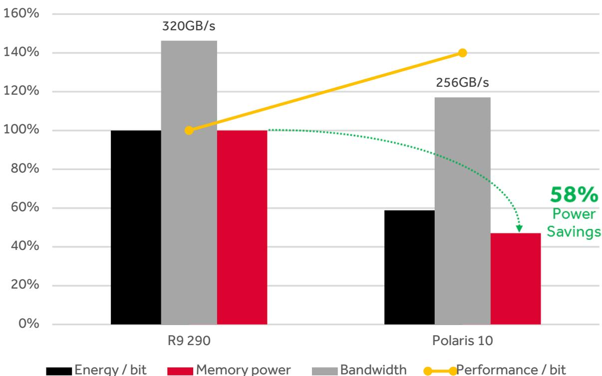
**Figure 8:** The Polaris architecture combines aggressive delta color compression, new buffers, and a larger L2 cache size to deliver higher performance/bit at 58% lower power than the Radeon™ R9 290 GPU (codenamed “Hawaii”).<sup>5</sup>
