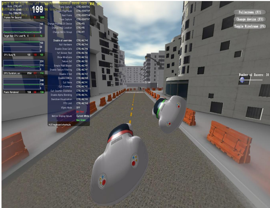
Figure 6: The head-up display (HUD) for Microsoft DirectX* workloads shows real-time metrics.
